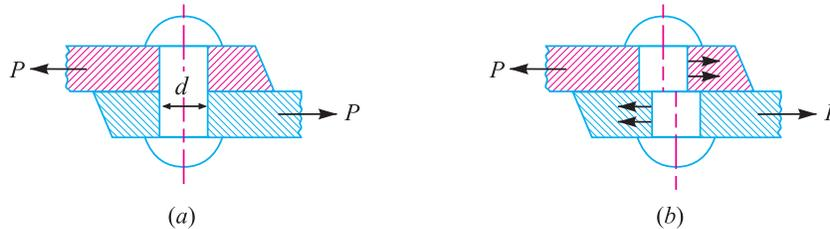
Fig. 4.6. Single shearing of a riveted joint.
