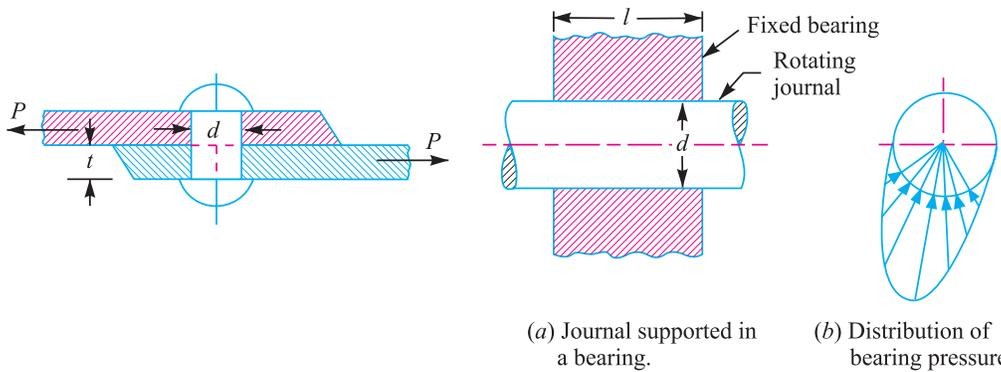
Fig. 4.9. Bearing stress in a riveted joint.
