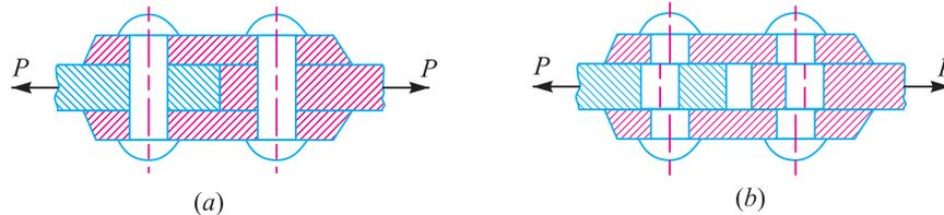
**Fig. 4.7.** Double shearing of a riveted joint.
